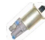
CLUTCH SERVO REF No.: WG9114230023 DIA: 90mm STROKE: 67mm AIR: M16x1.5 HYD: M14x1.5 APPLICATION: STR
