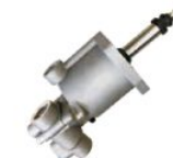
CLUTCH SERVO REF No.: 11-1602410-30 DIA: 100mm STROKE: 85mm AIR: M16x1.5 HYD: M14x1.5 APPLICATION: MAZ
