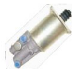
CLUTCH SERVO REF No.: WG9114230018/2 DIA: 102mm STROKE: 60mm AIR: M16x1.5 HYD: M14x1.5 APPLICATION: STR
