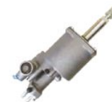
CLUTCH SERVO REF No.: 11-1602410-10 DIA: 100mm STROKE: 85mm AIR: M16x1.5 HYD: M14x1.5 APPLICATION: URAL
