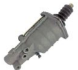
CLUTCH SERVO REF No.: VG3286AM DIA: 100mm STROKE: 85mm AIR: M16x1.5 HYD: M14x1.5 APPLICATION: IVECO
