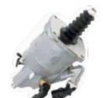
CLUTCH SERVO REF No.: 1000139593AM DIA: 100mm STROKE: AIR: M16x1.5 HYD: M14x1.5 APPLICATION: RENAULT
