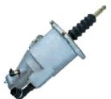
CLUTCH SERVO REF No.: 630361AM DIA: 100mm STROKE: 80mm AIR: M16x1.5 HYD: M14x1.5 APPLICATION: SCANIA
