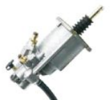
CLUTCH SERVO REF No.: 1000443297AM DIA: 100mm STROKE: 85mm AIR: M16x1.5 HYD: M14x1.5 APPLICATION: VOLVO
