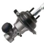
CLUTCH SERVO REF No.: 530100-1609510 DIA: 130mm STROKE: 35mm AIR: 1/8NPT HYD: M12x1.5 APPLICATION: KAMAZ
