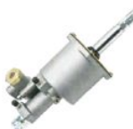
CLUTCH SERVO REF No.: 11-1602410-20 DIA: 100mm STROKE: 85mm AIR: M16x1.5 HYD: M14x1.5 APPLICATION: KRAZ, LIAZ, LAZ
