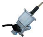
CLUTCH SERVO REF No.: 629276AM DIA: 100mm STROKE: 85mm AIR: M16x1.5 HYD: M14x1.5 APPLICATION: VOLVO
