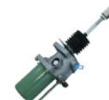
CLUTCH SERVO REF No.: APGA1605 DIA: 63.5mm STROKE: AIR: 1/8-27 UNF HYD: 7/16-20 UNF APPLICATION: DAF, VOLVO
